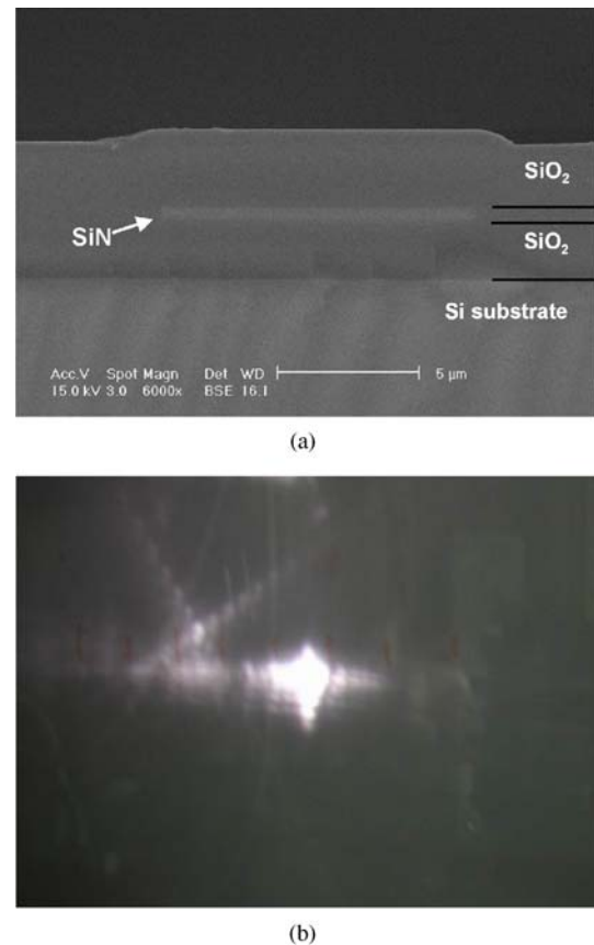
Fig. 5 The SiN optical waveguide (a) cross-sectional SEM images and (b) the input near-field output pattern shown on the display monitor of an infrared camera (mode image of straight waveguide)
